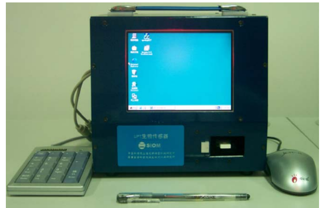
Fig. 2. Photograph of the portable prototype UPT-based biosensor.
