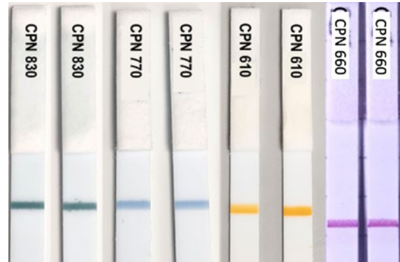
Figure 7 - Multi-coloured LFTs using CPN 830, CPN 770, CPN 610 & CPN 660 to detect ovalbumin
